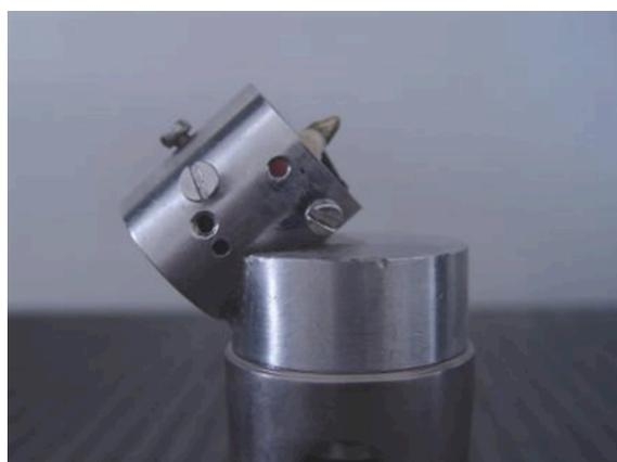
Figure 1. Tooth embedded in acrylic resin and correctly positioned into the metal device, before fracture resistance mechanical testing. The samples were angled at 45° to its base in the labial direction of the teeth.
