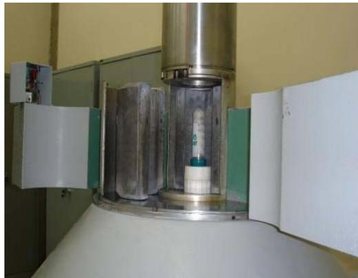
Figura 3: Fonte ( $^{60}\text{Co}$ ) Gamma Cell Atomic Energy
