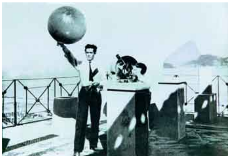
First aerological soundings with pilot balloons. The old terrace of the Meteorological and Astronomical Administration – Morro do Castelo.
